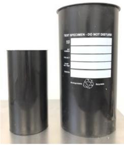
The strokes shall be distributed uniformly over the cross-section of the mould. The bottom layer shall be rodded throughout its depth. For the next two subsequent layers, the rod shall penetrate approximately 25 mm into the underlying layer. Tap the sides of the mould smartly 10 to 15 times if voids are left by the tamping rod to consolidate the concrete and to release any large air bubbles that might have been trapped.
