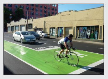
Bike Boxes are a new kind of street marking to help motorists and cyclists share the road. Bike boxes are used at intersections to designate a space for cyclists to wait in front of cars at a red light and then proceed first through the intersection when the light turns green. Once they clear the intersection they resume travelling in the bike lane.
