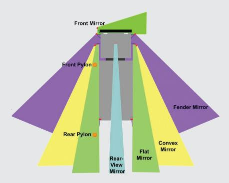
(Note: The rear view mirror shown here would not necessarily apply to Ready Mix trucks, however might apply to other vehicles in a Commercial Fleet.)
