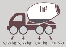
A proposed Seasonal Load Restriction of 6,500 kg/axle would allow a concrete truck to carry almost half it's load (4m3) reducing the number of trips to 2.
