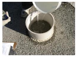
ASTM C1701 to evaluate the in-place infiltration rate of pervious pavement
