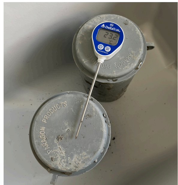
Figure 2: In-spec initial curing of concrete cylinders
